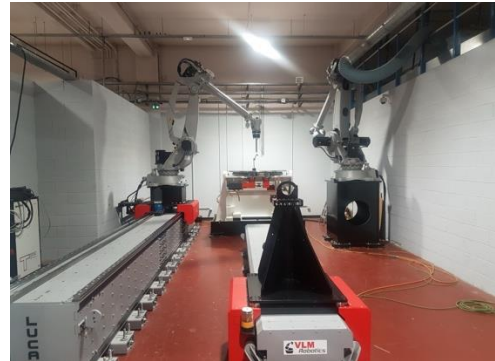
Version with one robot linear axis and one workpiece linear axis
