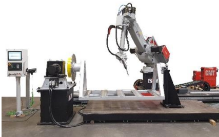
XXL machines: SOLO single robot or GEMINI bi-robot for parts up to 10m x 3m and 20 tonnes
